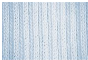
Fig. 4: Image of rib 2:2 finished knitted fabric
