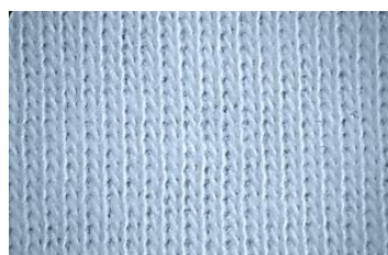
Fig. 2: Image of rib 1:1 finished knitted fabric
