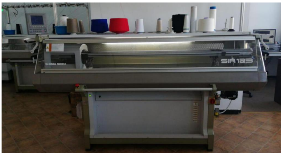
Fig. 5. The rectilinear knitting machine SHIMA SEIKI SIR 123 fineness 14
