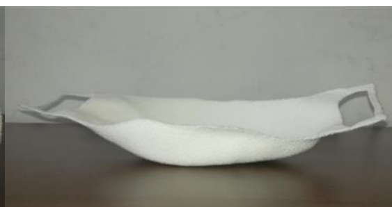
Fig. 7. Knitted protective mask - profile view
